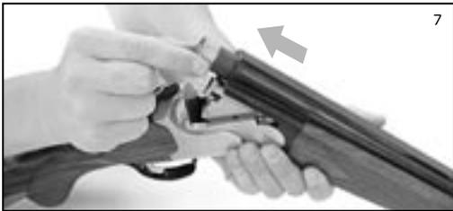
Once the breech is open and the shells removed the gun is safe. Remember to keep the breech open until you are ready to reload to prevent any mistakes or confusion as to the condition of the gun. If the breech is open anyone can see that the gun is unloaded.
