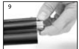
Care should be taken to ensure the keys on the wrench engage in the six large notches in the choke. Hold the gun tightly and unscrew the choke in a counter clockwise direction until it can be removed from the barrel.
