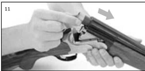
Point the shotgun in a safe direction and grasp the under side of the barrels at the front of the fore-end palm up and lift up smartly on the barrels while pushing down on the wrist of the stock. This action should cause the top lever to snap to the left slightly, locking the breech closed. (figure 12) Breech being closed.
